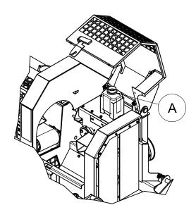
Ensure that the chain oil container does not drain during use. Also inspect that oil is consumed and the chain libricated..
