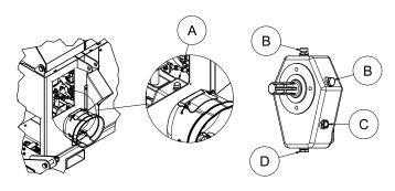
Check the oil level after each season by releasing level screw **C** as illustrated in the sketch (the oil to leak at sufficient level). Replacing oil via the breathing plug **B** on the top and the drainage via the plug **D**.
