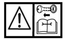
Before any sharpening work is initiated – stop the machine and tractor and remove the key to ensure unintentional start during the work
