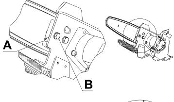
Inspect cutting chain and saw bar regularly. Sharpening ang tightening of the saw chain ensures effective cutting. Check that the vertical angle of the saw bar (90 degrees) so that the saw bar does not jam during cutting.
