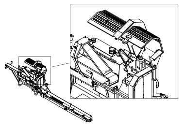
The covers over the chain bar and the cover over the splitting cradle can be opened as illustrated
