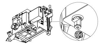
Regularly drain a small amount of hydraulic oil to check the oil quality. Grey oil is and indication of water in the oil caused by condensation Perform this inspection when the machines is cooled and eventual water concentrated at bottom level.
