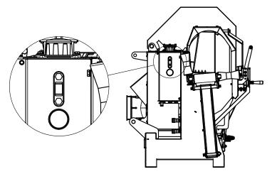
Inspect oil level and hydraulic oil temperature regularly. Refill oil if necessary Correct oil level should be in the middle of level glas when placed at horizontal level
