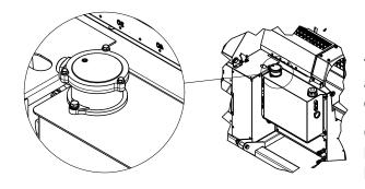
Replace the Filter cartridge in the oil filter after the first 50 operating hours, and afterwards once a year or after 500 operating hours (depending on whatever occurs first)
